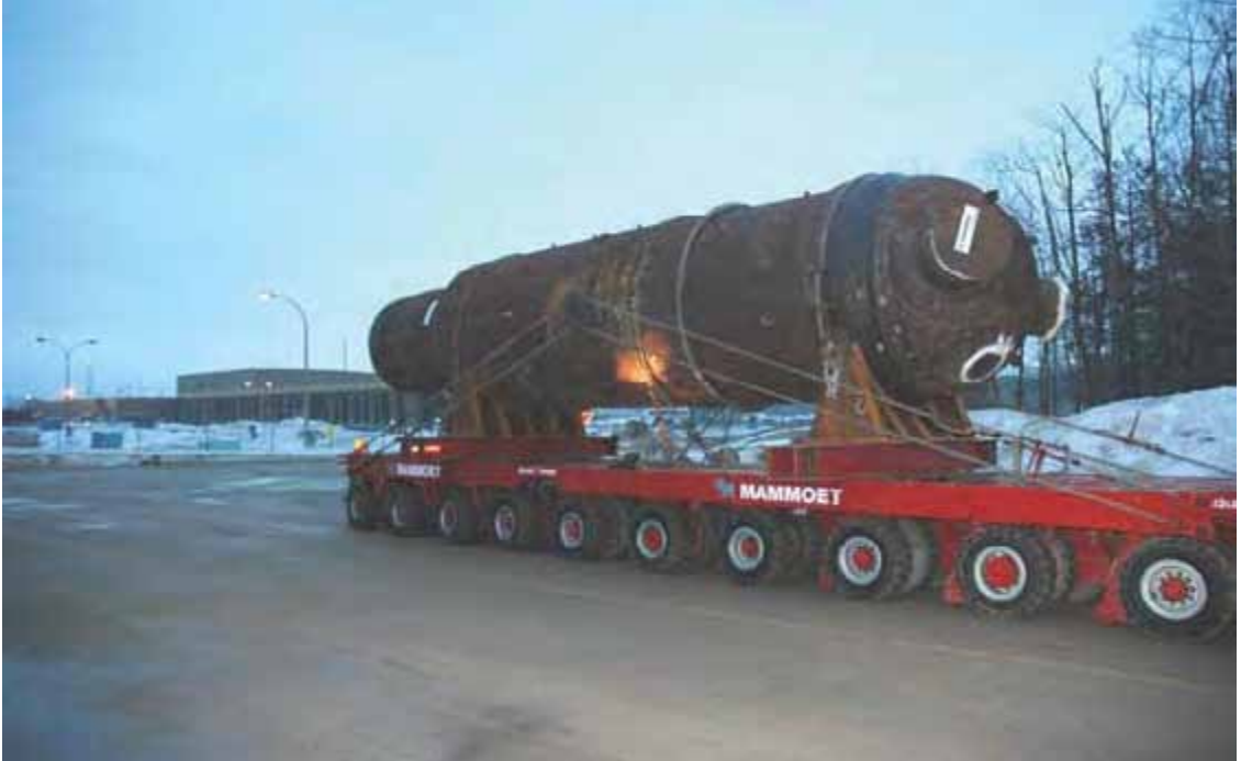
A steam generator is transported to the WWMF for interim management
